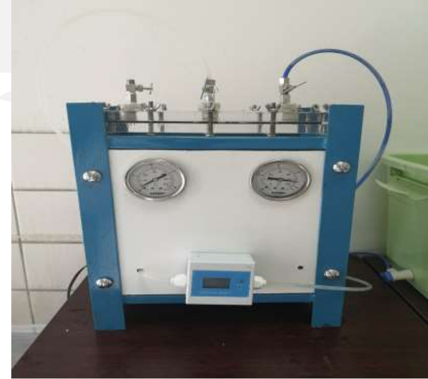
Figure : Membrane flat sheet tester (lab-scale)
