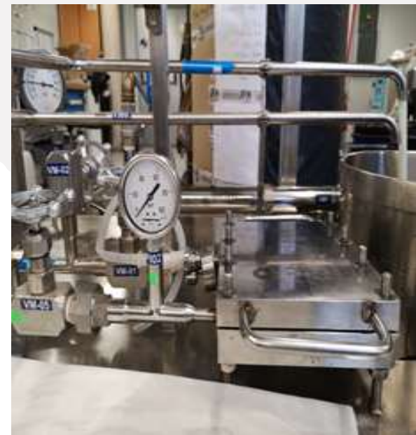
Figure 1 Tangential flow filtration system (cross flow) - IMDEA lab. Spain
