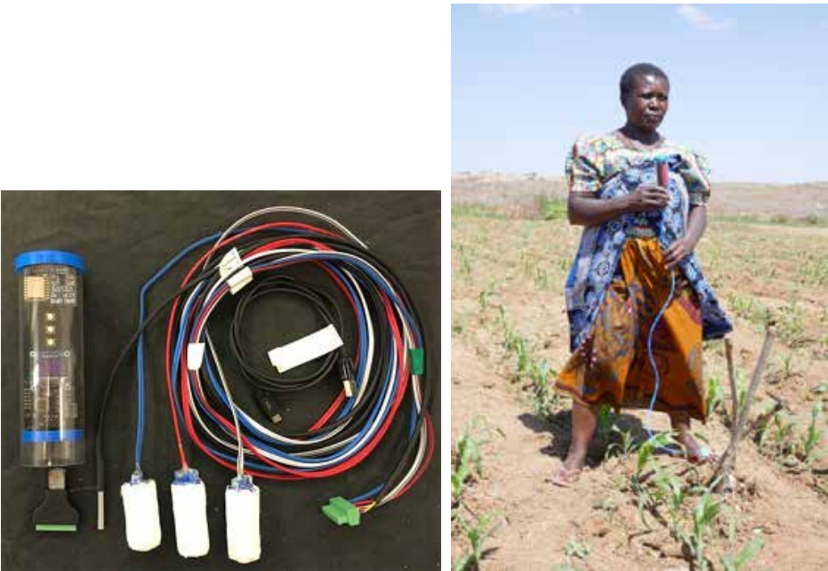
Figure 6. Chameleon™ soil moisture sensors and reader (Photo: VIA Farm website)
