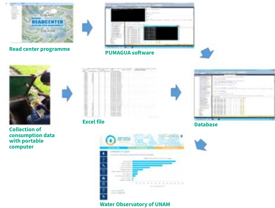
Figure 26. Integration of information to PUMAGUA database and to Water Observatory of UNAM from water meters linked to the remote system and from water meters that have not been linked yet.
