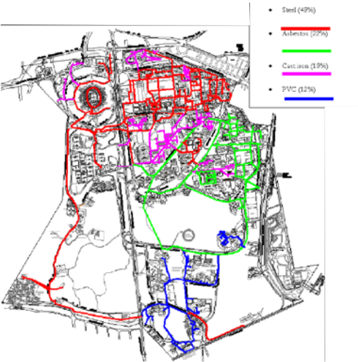
Figure 5. Digitalized water supply network of the University City of UNAM. Pipeline colours correspond to different materials: steel, asbestos, cast iron, and PVC. Source: PUMAGUA, 2012
