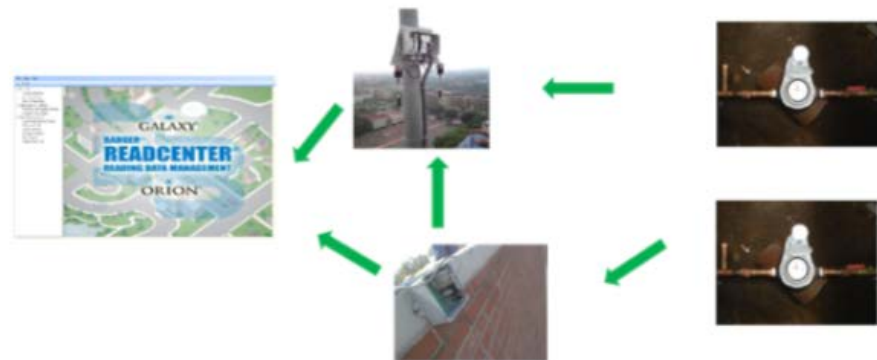
Figure 25. Direct and indirect transmission of water consumption information in the main campus of UNAM. Source: PUMAGUA, 2016
