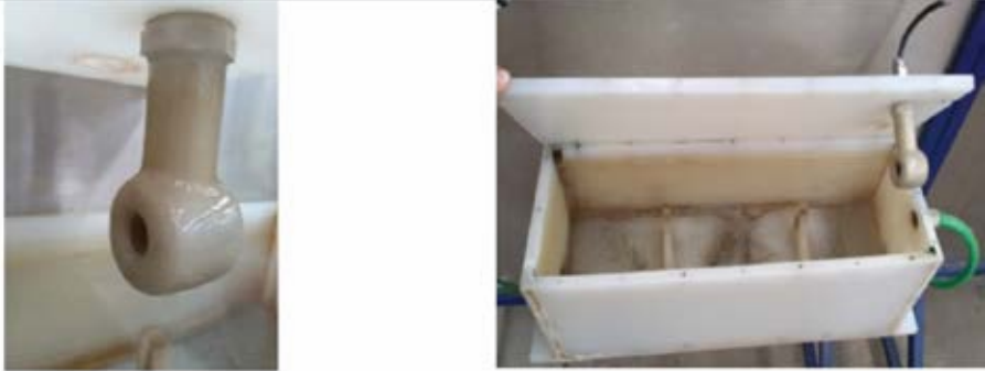
FIGURE 15. (A) Conductivity sensor of the real time water quality monitoring system; (B) a container was built to allow constant water flow. Source: Stephanie Espinosa, 2016.
