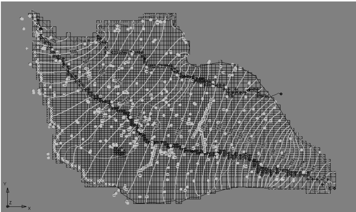
Figure 4. The regional groundwater flow model of the shallow Somes/Szamos alluvial transboundary aquifer.
